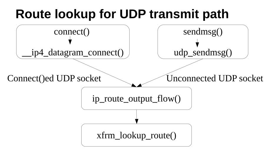
*ip\_route\_output\_flow() looks up the routing table via fib\_lookup() to find the path to the destination (aka "dst\_orig" in the code).* Then we look for any IPsec SPDs via xfrm\_lookup\_route(). Note that "XFRM" stands for IPsec transform
